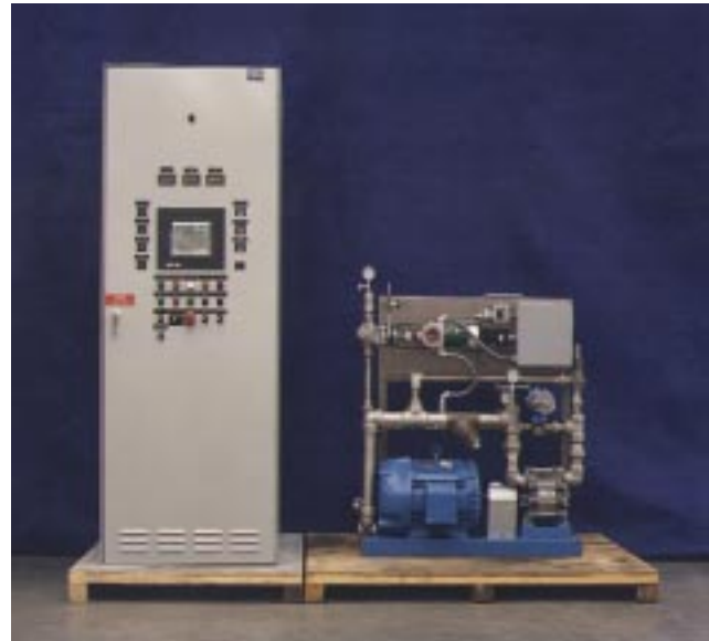
Replacement controls for one GE Frame 5 gen set in utility peaking service with water injection skid for NOx reduction
