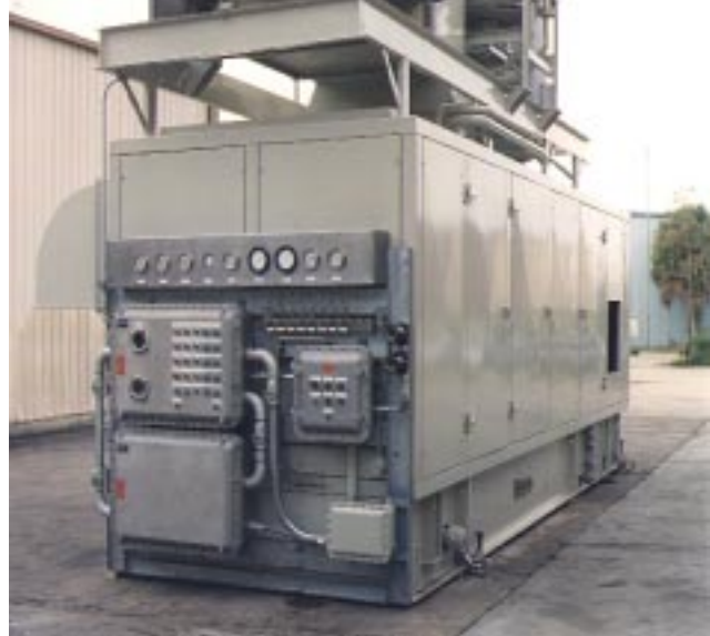
Explosion proof Division 2 replacement controls for Solar Centaur in offshore gas gathering service
